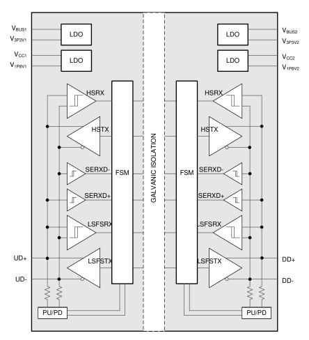
Figure 7-1. ISOUSB211-Q1 Simplified Functional Block Diagram
