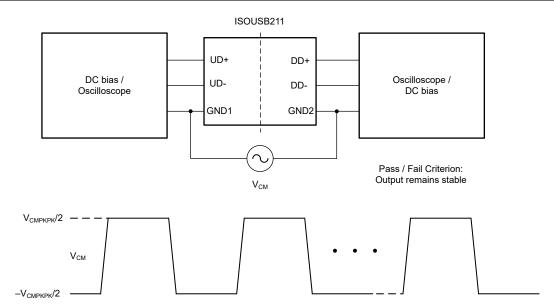
Figure 6-3. Common-Mode Transient Immunity Test Circuit
