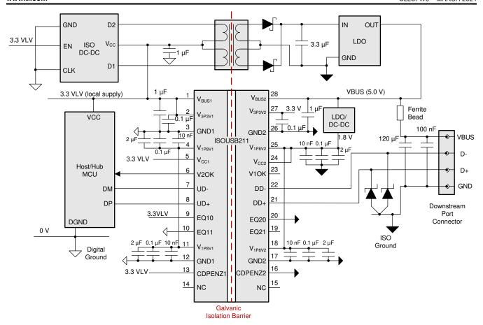
Figure 8-1. Isolated Host or Hub with ISOUSB211-Q1
