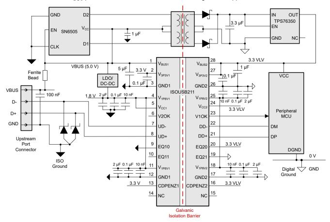
Figure 8-3. Isolated Bus-Powered Peripheral using ISOUSB211-Q1
