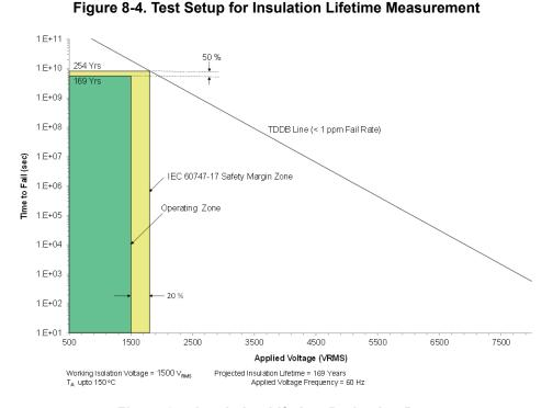
Figure 8-5. Insulation Lifetime Projection Data
