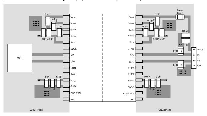
Figure 8-9. Layout Example for ISOUSB211-Q1
