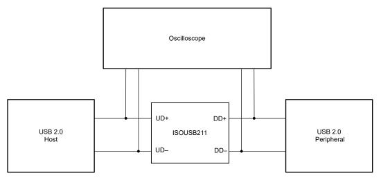
Figure 6-2. Upstream and Downstream Packet Parameter and Eye-Diagram Measurements for LS, FS
