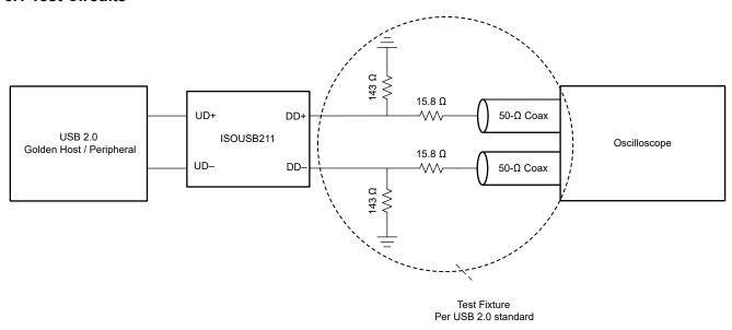
Figure 6-1. Upstream and Downstream Packet Parameter and Eye-Diagram Measurements for HS
