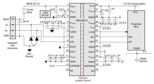
Figure 8-2. Isolated Self-Powered Peripheral with ISOUSB211-Q1
