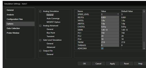
**Figure 4. Options tab of the Simulation Settings dialog**
